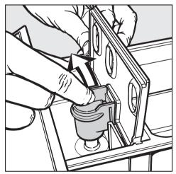
■ Remove the siphon tube from compartment <sup>®</sup>.
